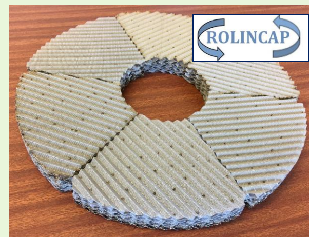
Montz structured packing (SS316) a_p = 830 \text{ m}^2 \text{ m}^{-3} \varepsilon = 0.94
