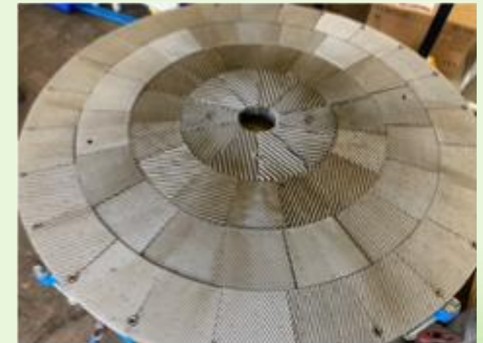
Variable porosity RPB packing from Montz
